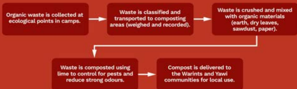
Figure 9. General composting process flowchart
